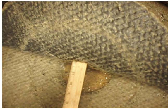
Figure 2. A test overlap showing bentonite “stain” on the surface of the woven geotextile, indicating extrusion from the non-woven.
