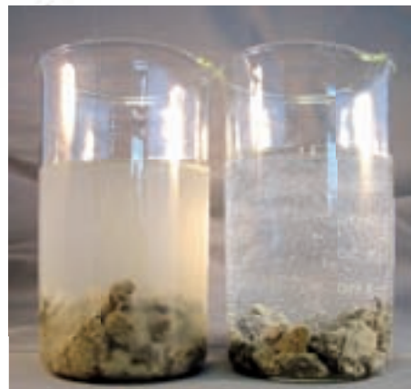
Wyoming sodium bentonite hydrating rapidly in tap water (left) and same product under control in high molecular weight polymer drilling additive (right)
