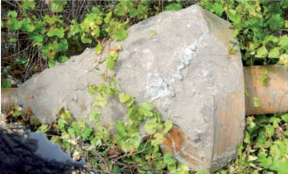
Above: a fluted reamer pack with clay
