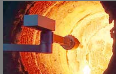
LaCam® LI Explorer – fixed installation With advanced technology for immersion of laser head, so gap and crack detection possible
