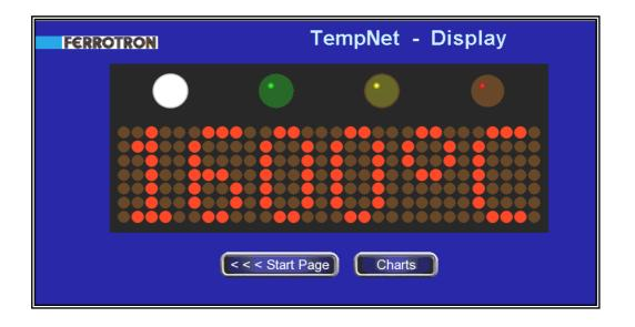
**Display** upper line - signal lights for indication of the measuring sequence lower line - result of temperature measuring
