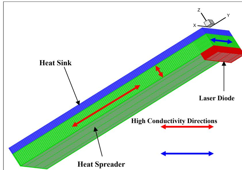
Finite control volume computational grid laser diode attached to the heat spreader
